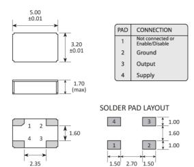
A 47nF ceramic capacitor must be connected between GND and VDD Dimensions in mm
