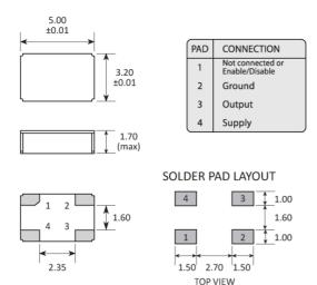
A 47nF ceramic capacitor must be connected between GND and VDD Dimensions in mm
