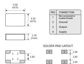
A 47nF ceramic capacitor must be connected between GND and VDD Dimensions in mm
