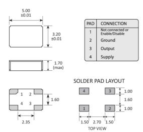
A 47nF ceramic capacitor must be connected between GND and  $\ensuremath{\mathsf{VDD}}$  Dimensions in mm
