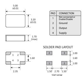
A 47nF ceramic capacitor must be connected between GND and  $\ensuremath{\mathsf{VDD}}$   $\ensuremath{\mathsf{Dimensions}}$  in mm
