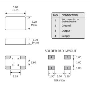
A 47nF ceramic capacitor must be connected between GND and VDD Dimensions in mm
