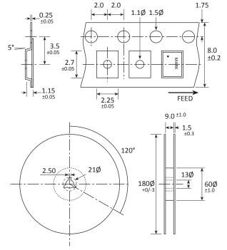
Not to scale. Dimensions in mm. Tolerances ±0.1mm unless otherwise stated
